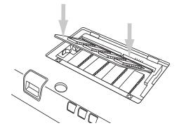
Figure 2-6 Installing a DIMM Module
